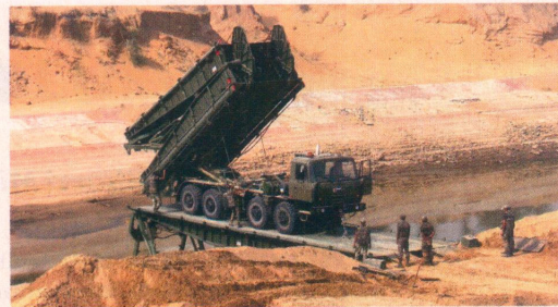
Bridging the Military Movement - BEML - Sarvatra Bridging System
