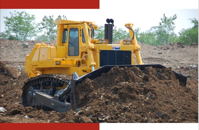
Flywheel horsepower (net) : 642 kW (860HP) @ 2000 rpm
