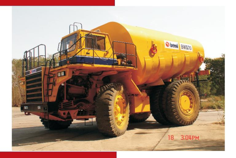
Flywheel power (net) : 674 kW (904HP) @ 2100 rpm
